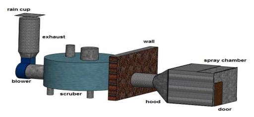
Fig. 2. The designed ventilation system, drawing by solid works 2014 software
