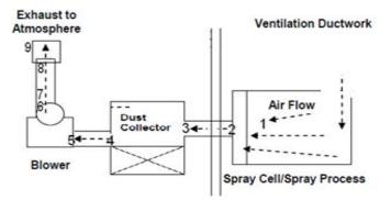
Fig.3. Critical points of the ventilation system
