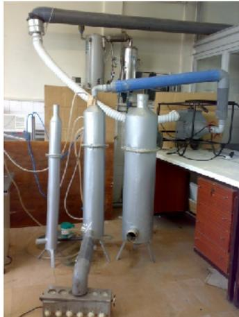
Fig 1. Packed towers used in the study
