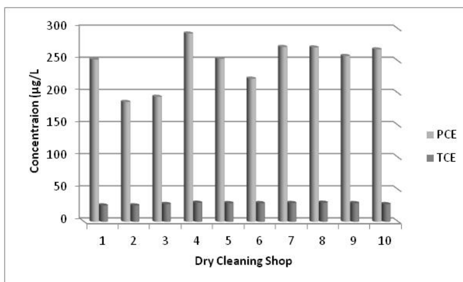
Fig 2. Mean PCE and TCE concentration in the effluents of dry cleaning shops
