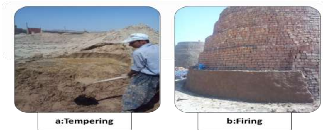
Fig 1. Image of Tempering (a) and Firing (b) steps in one of the brick workshops of Qom
