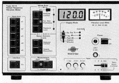
Fig 2. Human -Response Vibration Meter Type 2512 [14]
