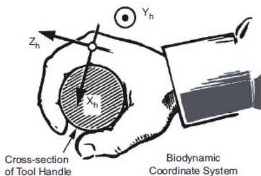
Fig 4. Axes of the acceleration components, ISO 5349-2001[22]
