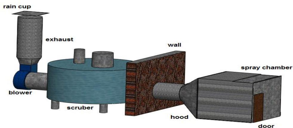
Fig. 2. The designed ventilation system, drawing by solid works 2014 software
