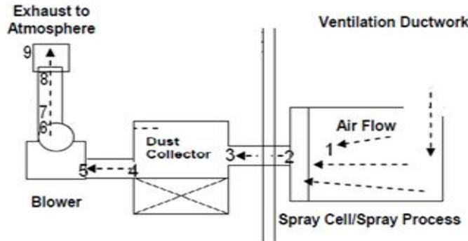
Fig.3. Critical points of the ventilation system
