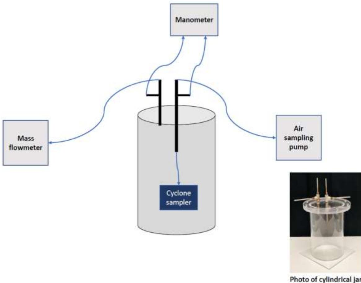
Fig 2. Schematic of design vessel
