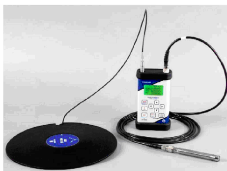
Fig 2. The view of the SVAN 948 instrument with the seat accelerometer, the preamplifier and the microphone
