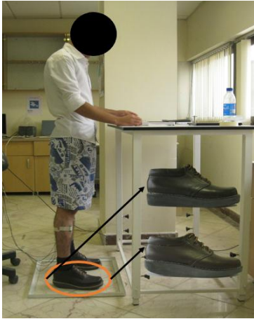
Fig. 1. Subjects standing for 2 h in each of footwear conditions while completing light assembly and mental tasks - Stable shoe (upper) and unstable shoe (lower) also illustrated here.
